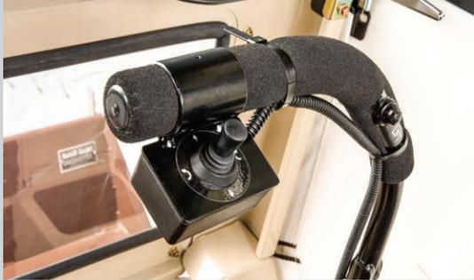
The optional Snow Performance Package increases productivity with on-the-go command of the implement. The joystick control, conveniently mounted to the steering lever, infinitely adjusts angles and height without leaving the operator's seat on the DriftBuster™ Snowthrower, CleanSweep™ bidirectional rotary broom and the Little Bully™ PowerBlade™.
