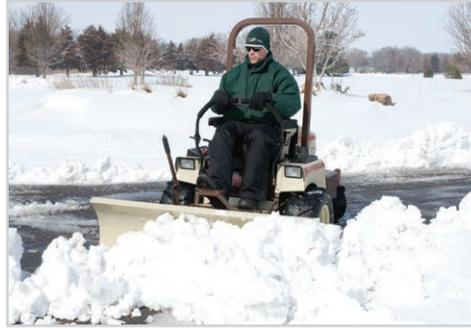
Multipurpose dozer blades offer unbelievable performance moving dirt, sand, gravel and snow. Blades operate straight ahead or 25 degrees left or right with manual pin positioning, and can be raised and lowered with hand or foot controls for easy operation, responsive control and timesaving efficiency.
