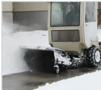
PTO-driven rotary brooms sweep dirt and debris, and clean up to 8 inches of snow. Only 1/2-3/4-throttle is necessary for optimum efficiency. Fixed-angle models sweep at a 25-degree angle to the right. The bidirectional broom angles 25 degrees left or right to fit your application.
