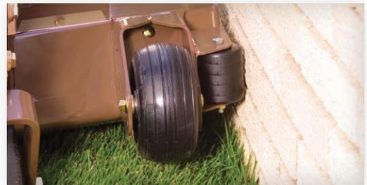
SpeedTrimming™ Heavy-Duty Roller Kit
