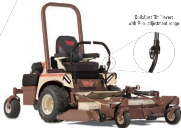
QuikAdjust Tilt™ levers with 9-in. adjustment range
